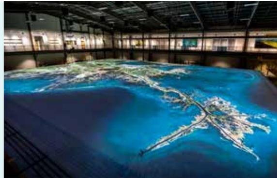
The Lower Mississippi River Physical Model simulates the river's depth, sediment and flow and is designed to study how it responds to modification. Twenty high-resolution projectors are mounted above the model bed to project aerial photographs, project features, diversion outputs and other simulations/animations.
